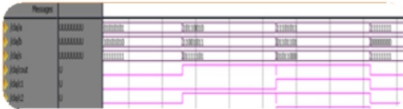
Fig.8. shows carry look ahead adder output waveforms
