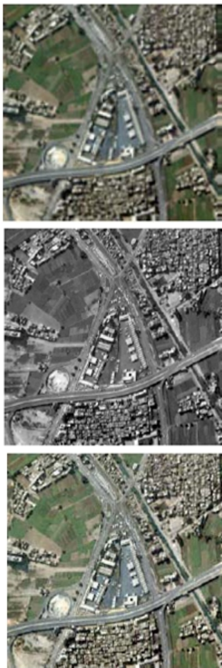
Fig. 1.1. Image fusion for an IKONOS scene for Cairo, Egypt: (a) multispectral low resolution input image, (b) panchromatic high resolution input image, and (c) fused image of IHS.
