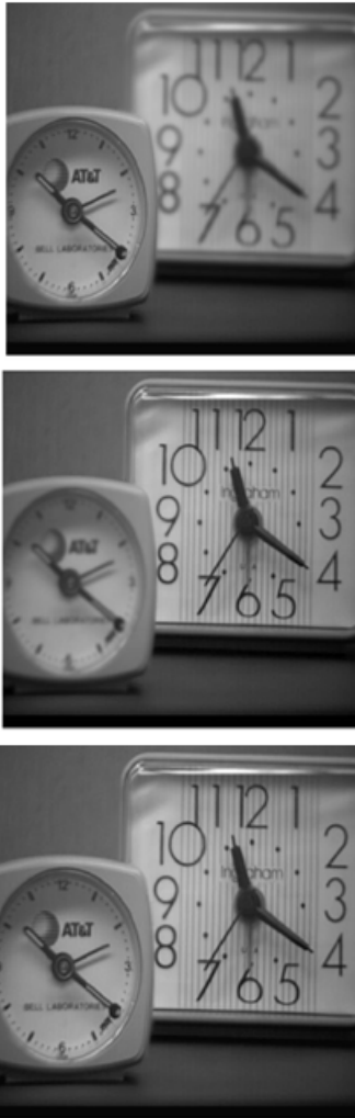
Fig. 1.2. CCD visual images with the (a) right and (b) left clocks out of focus, respectively; (c) the resulting fused image from (a) and (b) with the two clocks in focus.
