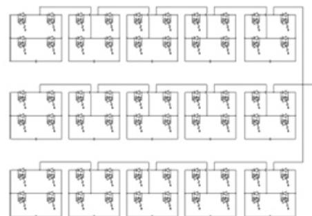
**Fig. 1. Eleven-level cascaded multilevel STATCOM.**
