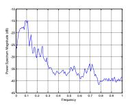
Simulation results for echo cancellation using FastAdaptive Kalman filter algorithm for speech as input
