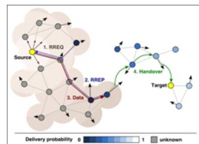
**Fig.1. Example of Mobile-Adhoc Network**
