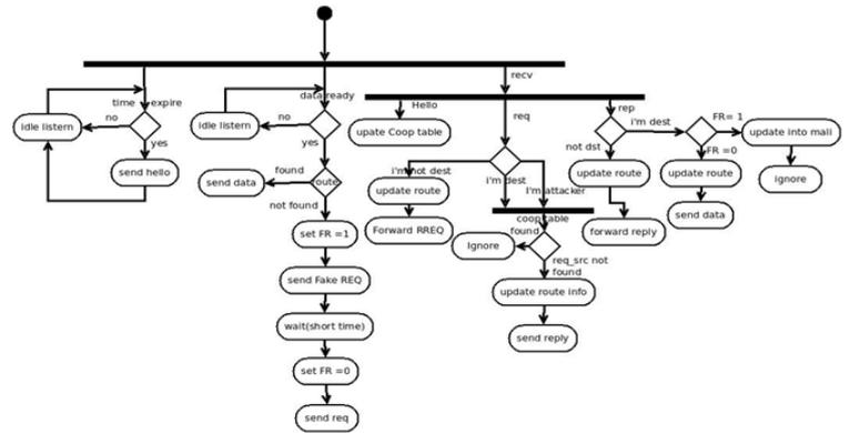
**Fig.4. activity of coop bait detection system**
