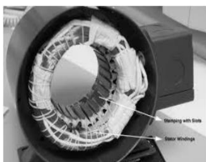
Fig.1 BLDC motor stator construction
