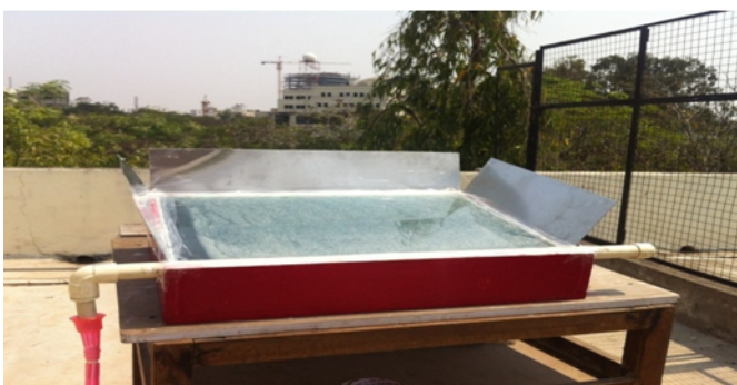
fig.1.3: solar still with required size of aluminum sheet
