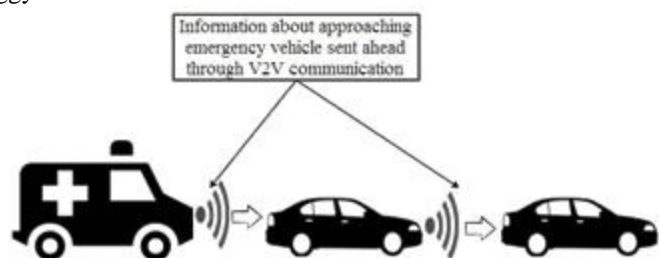
Fig. 6: Approaching emergency vehicle warning
