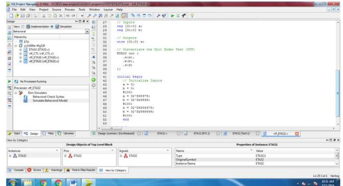
**Fig 8. Test Bench of 32bit error-tolerant adder (ETA)**
