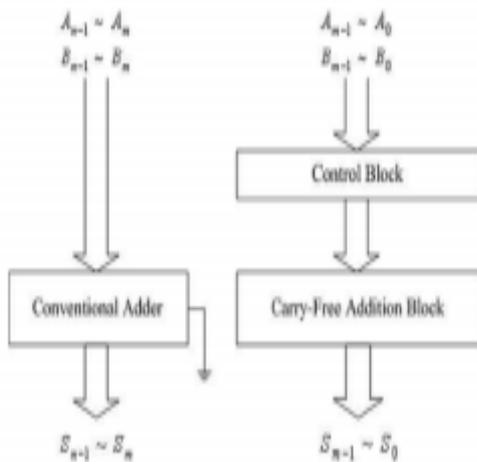
Figure.1: low power high speed error tolerant adder
