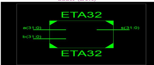
**Fig 6. Technology schematic of 32bit error-tolerant adder (ETA)**
