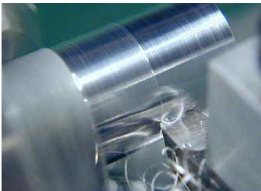
Fig 3:turning with power feed
