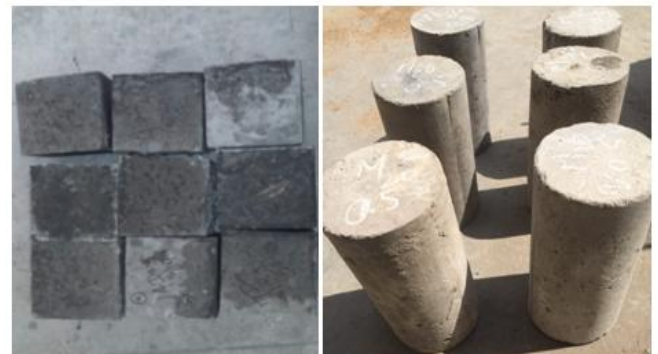
Fig 4.4 Casted concrete cubes and cylinder
