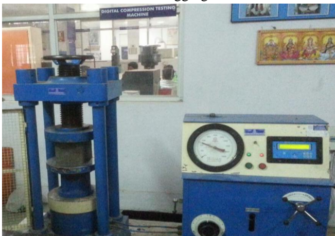
Fig 4.6 Compression testing of Specimen
