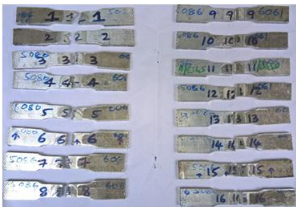
Fig 7: specimens after braking under UTM tension test
