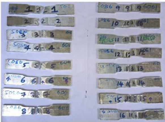
Fig 6:specimen failed under tension at peak load point
