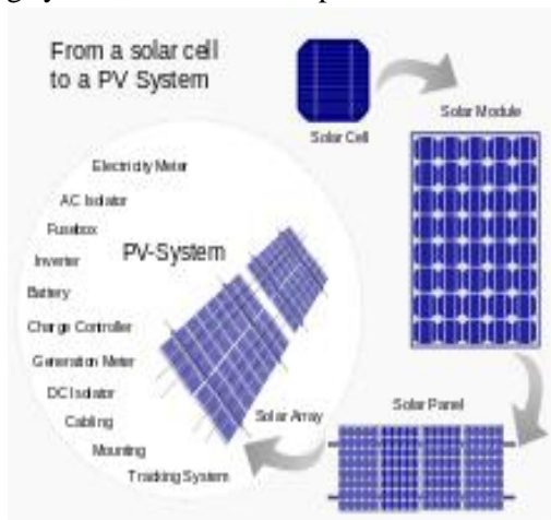
Diagram of the possible components of a photovoltaic system.
