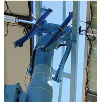
A 1998 model of a passive solar tracker, viewed from underneath.
