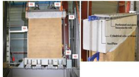
Fig. 2. (a) Test setup on a RE wall ( 1.5\text{ m} \times 1.5\text{ m} \times 0.25\text{ m} ), (b) System placed on top of the beam.
