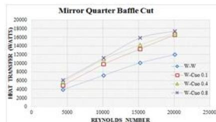
Figure.16 Heat transfer at different working fluids with mirror quarter baffle cut
