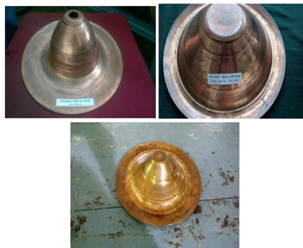
Fig. 10- Experimentally spun samples by using different CNC roller paths
