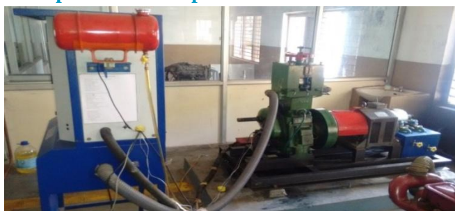
Fig 4.1: Computerized VCR Engine Test Rig
