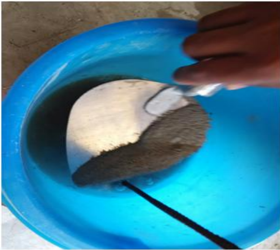
Figure 4: Adding some amount of cement, silica fumes mix
