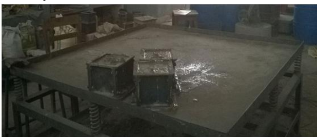
Figure 6: Placing the concrete filled moulds on vibrating machine
