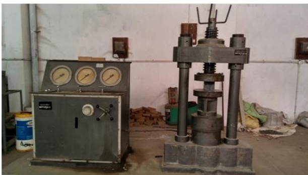
Figure 9: Compressive testing machine
