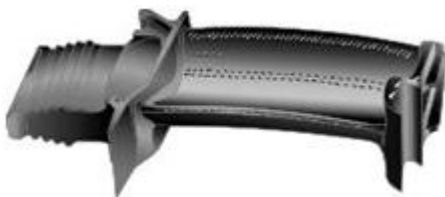
Fig1: Diagram of a high-pressure film cooled turbine blade
