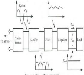
Components of a typical linear power supply
