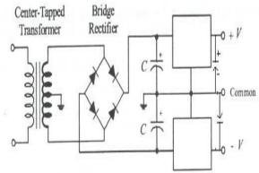
A regulated power supply essentially consists of an ordinary power supply and a voltage regulating device, as illustrated in the figure. The output from an ordinary power supply is fed to the voltage regulating device that provides the final output. The output voltage remains constant irrespective of variations in the ac input voltage or variations in output (or load) current.
