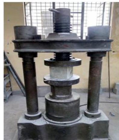
Fig.4.1. Compressive Strength Test on Concrete Cube
