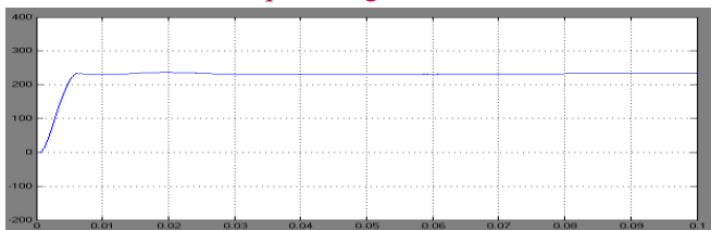
Figure 15: Converter DC voltage under operating condition using PWM
