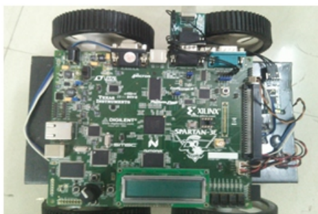
Figure2: Interfacing of FPGA to robot.
