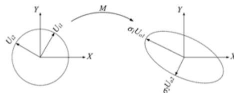
Fig. 2. Concept of the SVD of a matrix.
