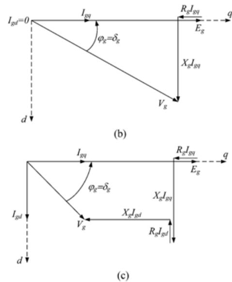
Fig. 10. Phasor diagram of PMSG for different values of  $I_{gd}$ . (a) PMSG equivalent circuit. (b)  $I_{gd}=0$  (c)  $I_{gd}>0$
