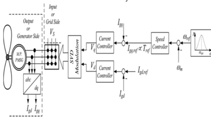
Fig. 9. Simplified control block diagram of a PMSG.
