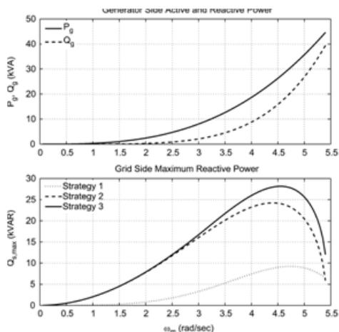
**Fig. 11. Generator-side active and reactive power and the maximum grid side reactive power versus generator shaft speed  $\omega_m$  for different strategies.**
