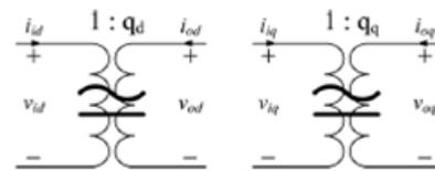
Fig. 4. Matrix converter steady-state and dynamic  $d_q$  transformer model.
