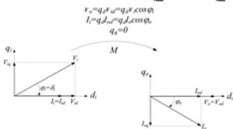
Fig. 6. Modeling the SVM modulation method by the SVD modulation technique
