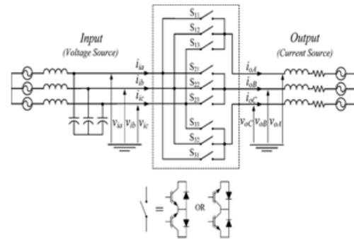
**Fig. 1. Typical three-phase matrix converter schematic.**
