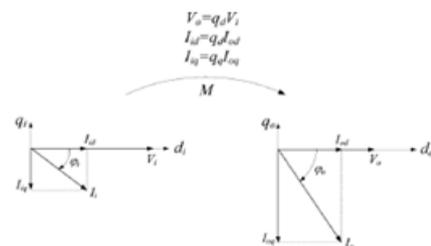
Fig. 5. Modeling of Alesina and Venturini modulation method by the SVD modulation technique.
