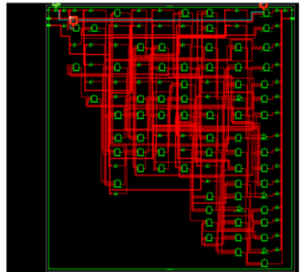
Fig9: Technology Schematic of 16bit-BK-BEC Carry select adder
