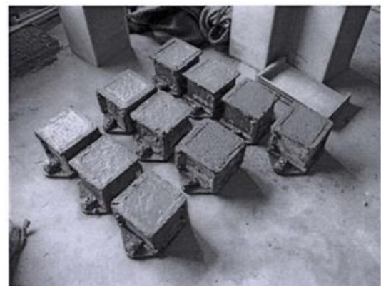
Figure 3.2 the cubes cast for the cube tests
