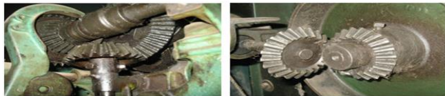
Fig 6: Straight level Gears Mounted on shafts: Left-on loom; Right-on Carding Machine.
