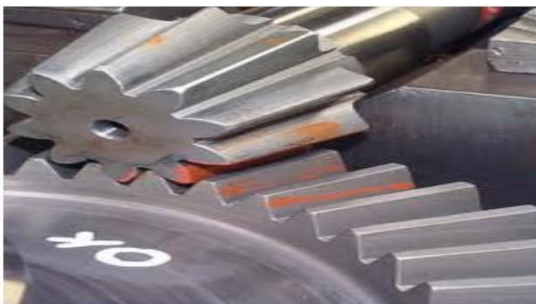
Fig 11: Angular bevel gears (Angle of separation >90^\circ )
