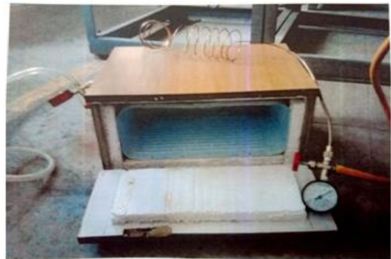
Fig 7: Evaporator with insulation
