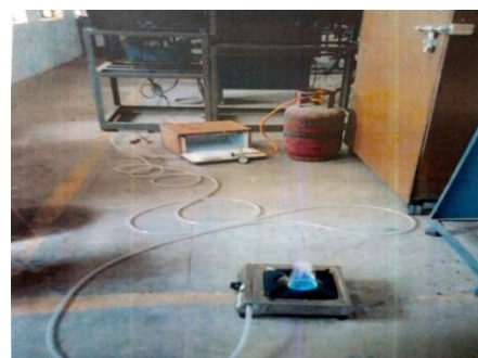
Fig 11: LPG refrigeration and heating system
