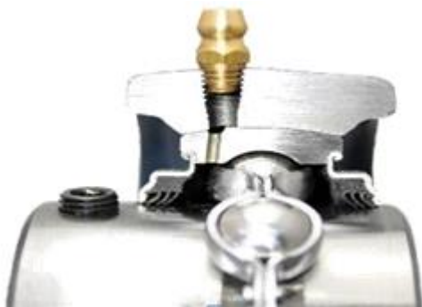
Fig4: typical pillow block bearing lubrication
