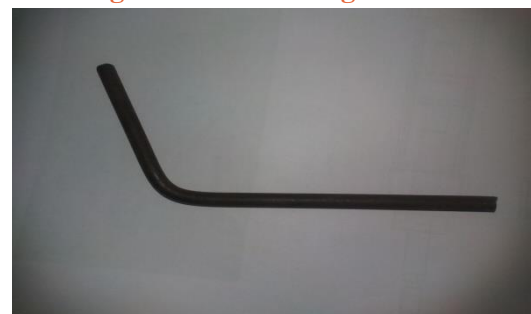
Fig 10: After bending of a rod(45°)
