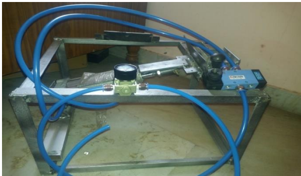
Fig 6: Machine diagram of a pneumatic bending machine
