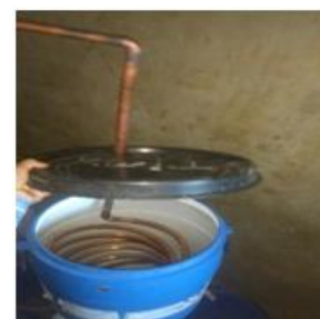
Fig.8.2 Helical coil Heat exchanger with casing
