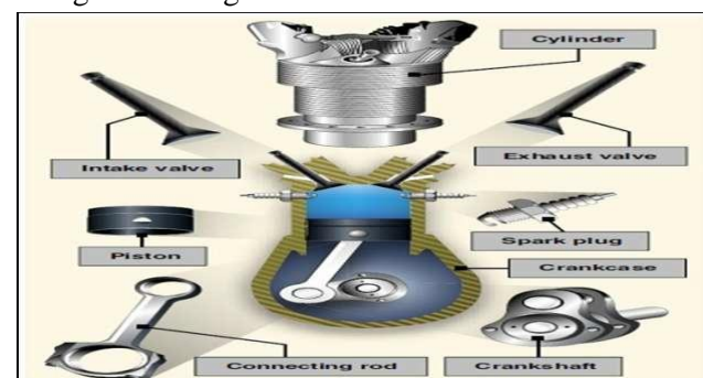
Fig.1.1 Main components of spark ignition reciprocating engine
