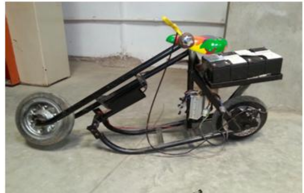
Fig 10: Modified frame folded
