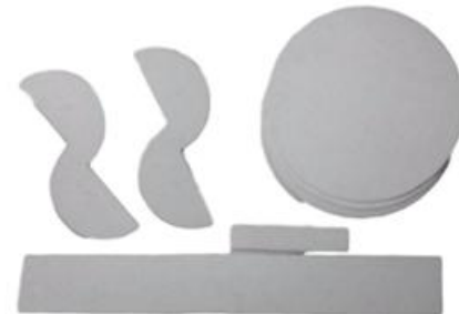
Fig. 3.17 Cutting of Depron sheets into required shapes
