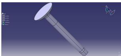
Fig 3.2 CATIA model of bi metallic valve
