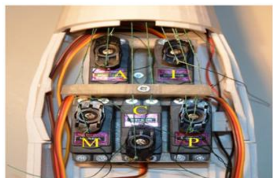
Fig 3: Top view of the servos, marked with the initial finger control
