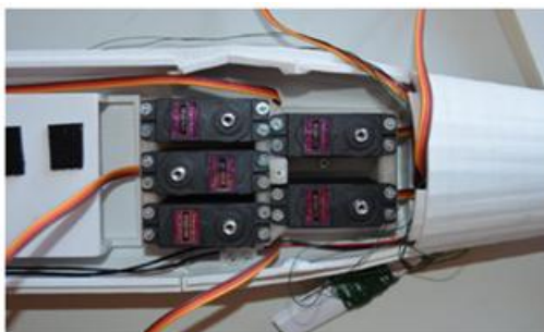
Fig 8: Servos mounted on its support on the forearm
