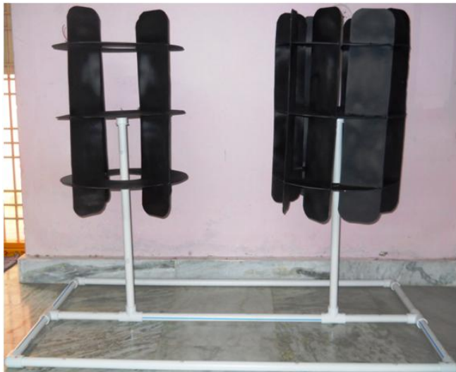
Fig. 19 Assembling of 4B & 8B VAWTS
