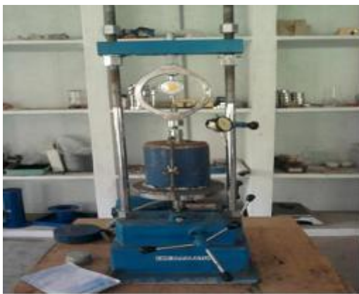
Fig.4 California Bearing Ratio Test
