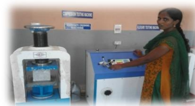
Fig. 2: Compressive strength testing machine
