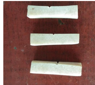
Figure 7: Specimen shown for Impact Test
