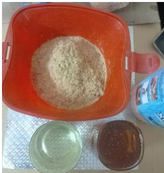
Figure 4: Epoxy resin, hardener & shrimppowder
