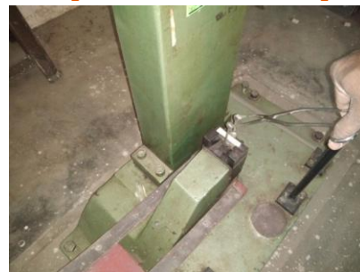
Figure 8: Specimen shown for impact test.
