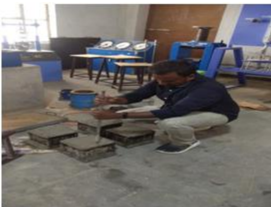
Casting of Moulds
