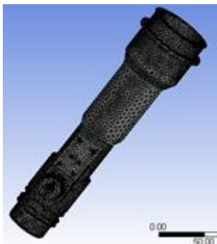
Fig. 2. Mathematical model of injector body
