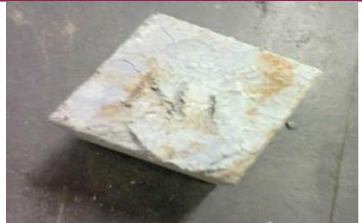
Fig.5.8.Specimen of HSVC after heating to 600 0 C at 6hr duration
