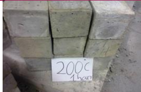
Fig.5.2.Specimens after heating 200 0 C at 1hr duration
