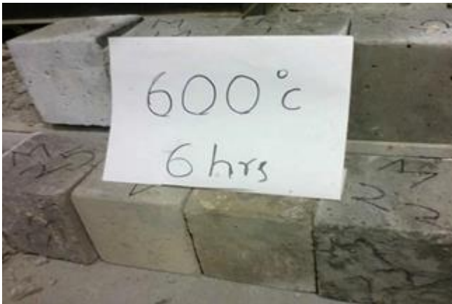
Fig5.6.Specimens after heating 600 0 C at 6hr duration
