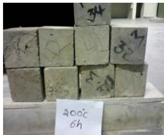
Fig.5.3.Specimens after heating 200 0 CC at 6hr duration
