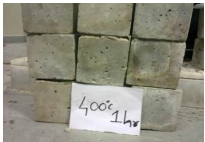
Fig.5.4.Specimens after heating 400 0 C at 1hr duration
