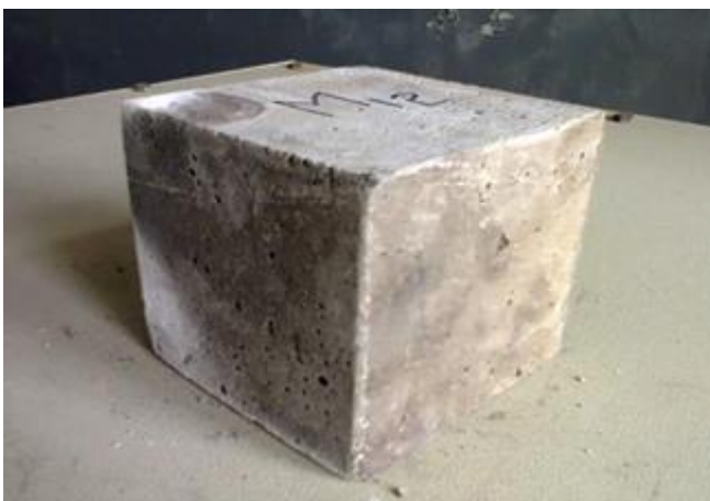
Fig 5.7.Specimen of M12 after heating to 600 0 C at 6 hr duration.
