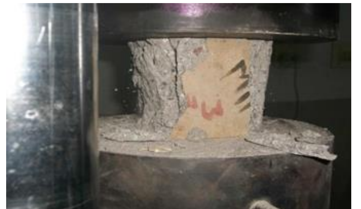
Fig.5.9.Specimen of HSSCC while testing after heating to 400 0 C at 6hr duration
