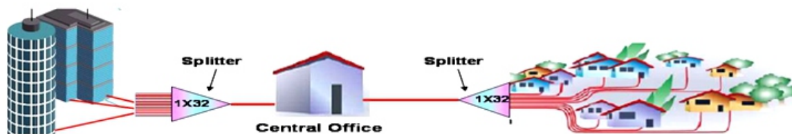
Fig. 7 Centralized Splitter Approach
