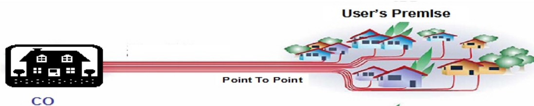
Fig. 4 Home Run Fiber (Point-to-Point) architecture
