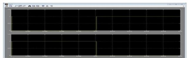
Fig.6. PWM signals for S2 and S4.
