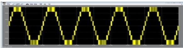
Fig.9. Inverter output voltage.
