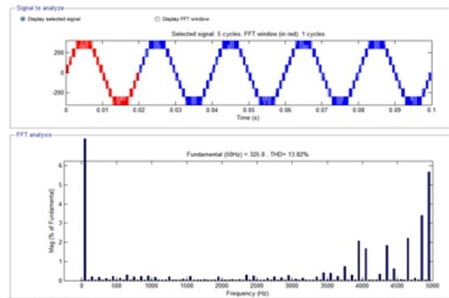
FIG: FFT for nine level Inverter.
