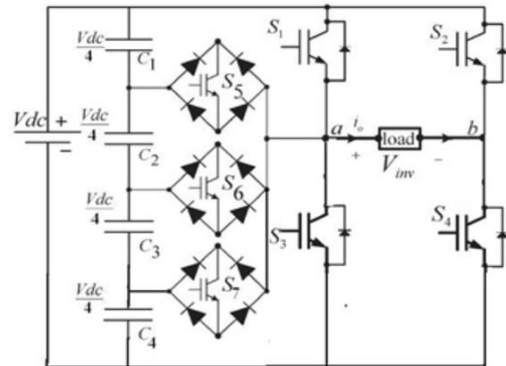
Fig. 2. Nine-level inverter for switching operation.
