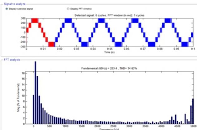
FIG: FFT for seven level Inverter.
