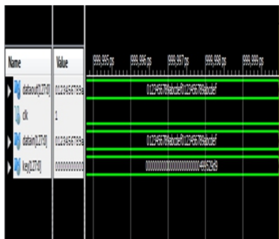
Figure-6: Simulation waveform of 128 bit AES (Decryption)
