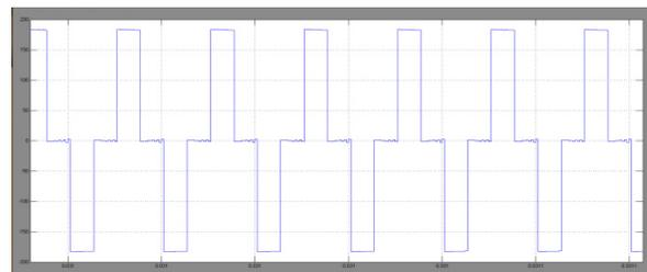
**Fig.11: Three Level Output Voltage**
