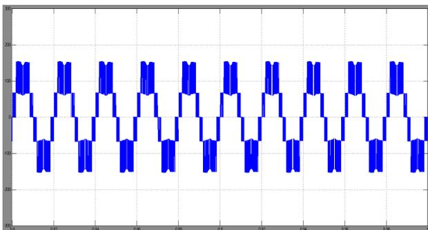
**Fig.11. five level output at primary side of transformer**
