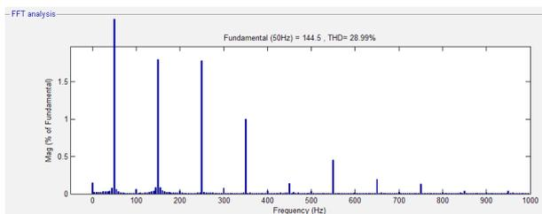
**Fig.12.FFT window for five level output at primary side of transformer**
