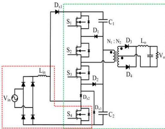
Fig.1. Proposed single-stage three-level converter.
