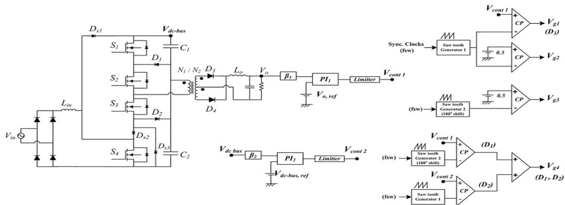
Fig.4 Simplified schematic control of the proposed converter of the converter can be made to operate in an optimal manner.
