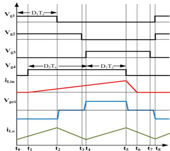
Fig. 2. Typical waveforms describing the modes of operation.
