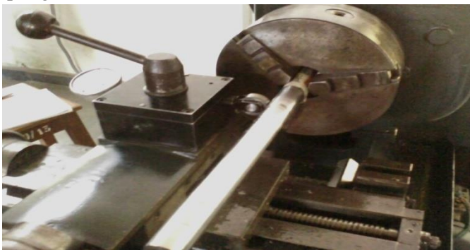
Fig. Burnishing process performed on specimen.
