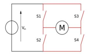
The two basic states of a H-bridge. The term "H-bridge" is derived from the typical graphical representation of such a circuit. An H-bridge is built with four switches (solid-state or mechanical). When the switches S1 and S4 (according to the first figure) are closed (and S2 and S3 are open) a positive voltage will be applied across the motor. By opening S1 and S4 switches and closing S2 and S3 switches, this voltage is reversed, allowing reverse operation of the motor.
