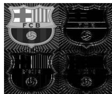
Fig 4.1.10 One-Level Decomposition of Watermark Image Using Haar DWT
