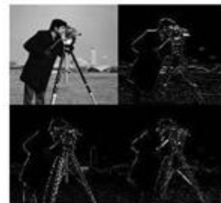
Fig 4.1.9 One-Level Decomposition of Original Image Using Haar DWT
